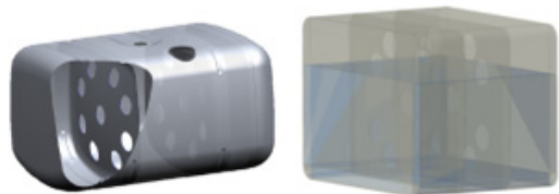
Fig. 14 (a) Baffle shape with prismatic tank (b) FE model with baffles
